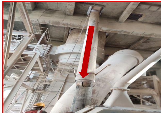
Avoided running of belt conveyor 362BC4 by providing direct chute modification at separator discharge
